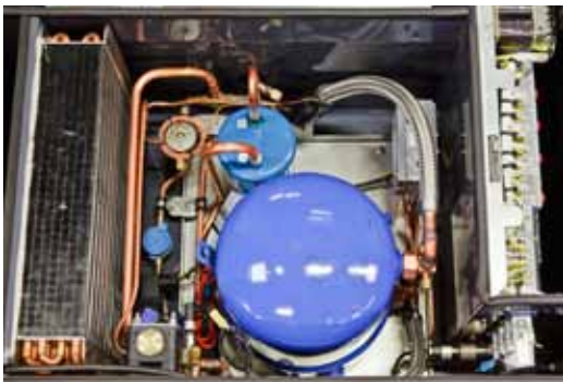
Compressor/Condenser for air-conditioning unit
